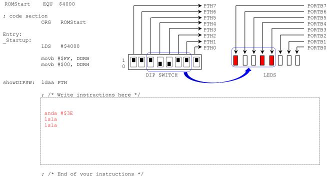
staa PORTB ; Contents of register A are written on PORTB bra showDIPSW • (5 pts) What is the time delay (in ms) that the following loop generates? Assume a 25 MHz bus clock. Consider that pusha takes 2 cycles, pula 3 cycles, nop one cycle and dbne 3 cycles.
